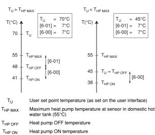
NOTE T<sub>HP MAX</sub> is a theoretical value. In reality the maximum tank temperature that can be reached with the heat pump is 53°C. It is advised to select T<sub>HP OFF</sub> not higher than 48°C in order to improve performance of the heat pump during domestic water heating mode.
